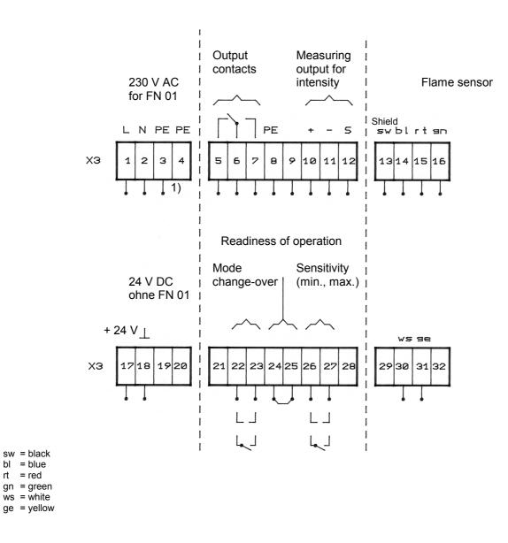
1) it's always necessary to connect ground clamp
