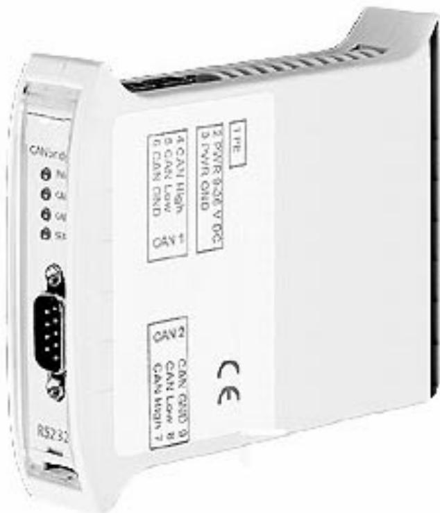
The CANbridge is used for coupling the LAMTEC SYSTEM BUS at CANopen. Thereby it will be possible to receive and evaluate boiler datas from GESTRA.
