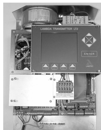
Without reference air pump: Type 657 R 1028 400 x 300 x 150 (HWD)
