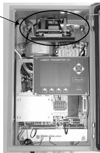
With reference air pump: Type 657 R 1060 When the optional reference air pump is used, the size of the wall-mounted housing changes 500 x 300 x 200 (HWD)
