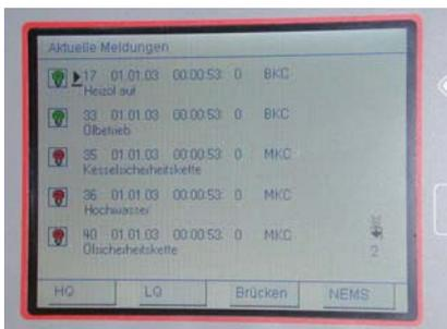
For displaying incoming and outgoing fault and process status signals in chronological order. Timing accuracy of the time stamps: typ. + 1 ms, max. + 5 ms.
