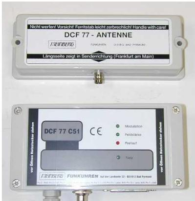
The system time can also be sent to the system via a radio clock connected to the 2<sup>nd</sup> RS232 port instead of the integrated real-time clock.
