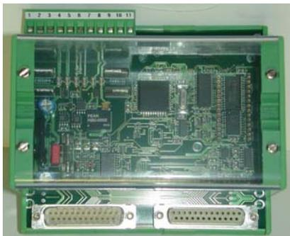
The NEMS signals can be converted to a standard field bus protocol (Profibus, Interbus-S, CAN-Open, Modbus, Ethernet) via a communications processor connected to the LAMTEC SYSTEM BUS.
