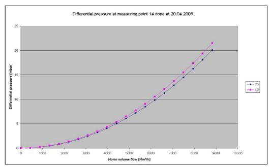
The software for calculation computes particularly for each size the differential pressure curve. For this must lattice geometry, measuring range, measuring medium (density), temperature and system pressure admit to be.
