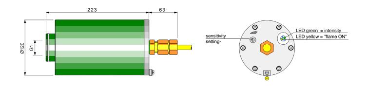
Class: EEx d IIC T 6 for PTB 87/1095
